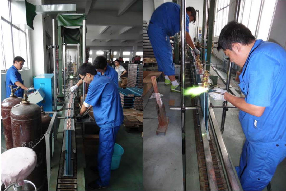
Tube soldering by automat machine and pipe soldering by worker well
