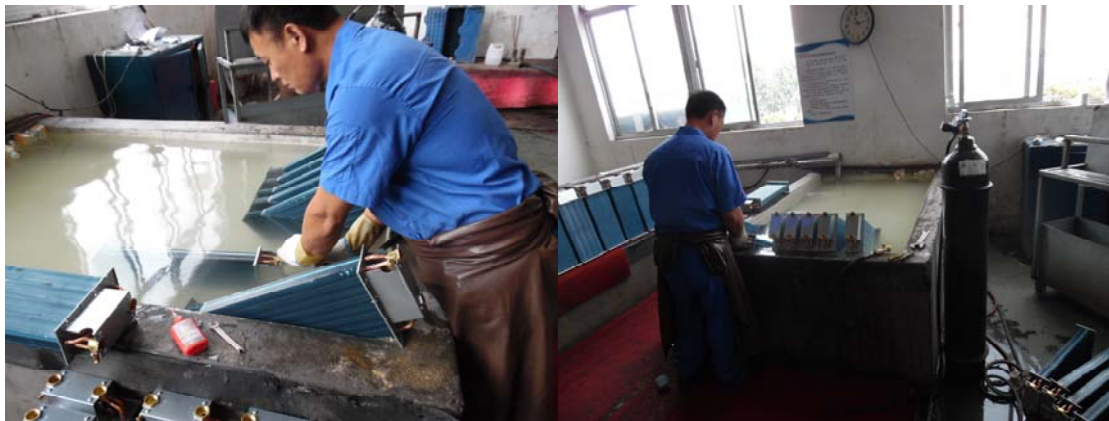
Tube soldering by automat machine and pipe soldering by worker well
