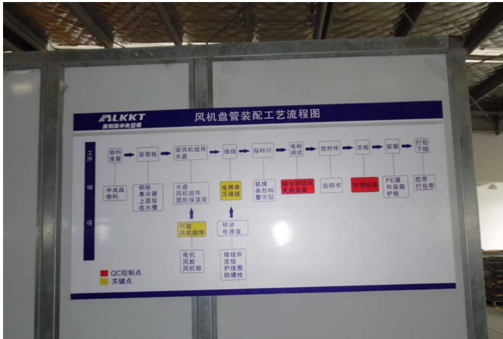
Fan coil producing progress flow chart.
