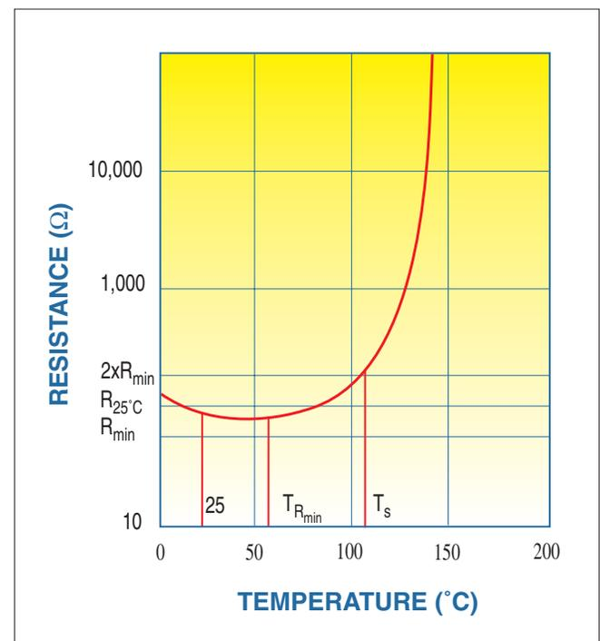
Figure 12: Resistance versus Temperature for a PTC
